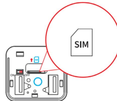
When the nano SIM card is inserted and the AM-T01 is ON, the LED will light up.
