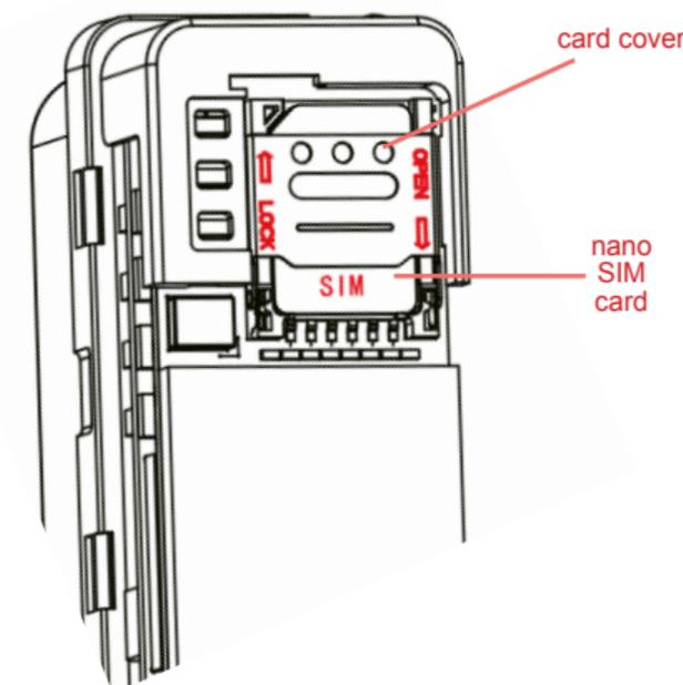
When the nano SIM card has been inserted the AM-T22 will use the fitted backup battery. If this is not charged, please connect to the vehicle's OBD socket to recharge.
